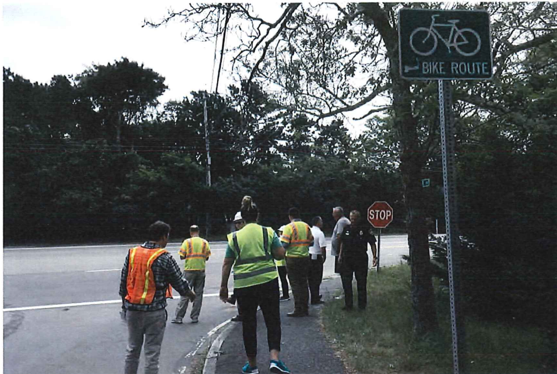
Figure 13 - Aspinet Road approach showing low stop sign and ambiguous bike route sign
